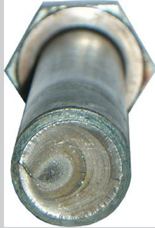
Fig. 1 — Bending fatigue failure (source: Bolt Science).
