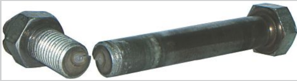
Fig. 2 — Bending fatigue failure (source: Bolt Science).
