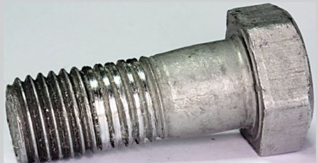
Fig. 5 — Thread stripping of a galvanized bolt (source: Bolt Science).
