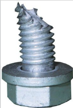
Fig. 4 — Bolt overload failure (source: Bolt Science).
