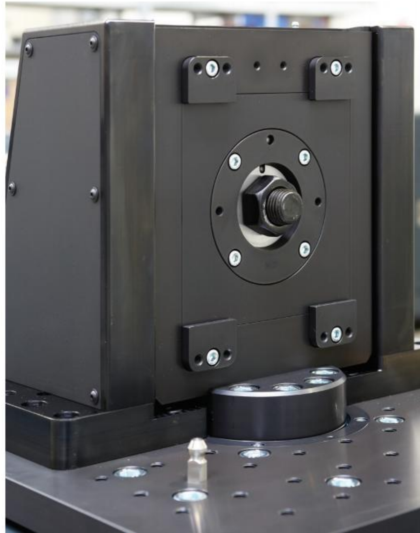
Figure 2: Junker test fixture using roller bearings between clamped parts. Although ideal for comparing fastener locking element performance, the fixture materials have different inner joint surface friction characteristics than those specified in the bolted joint design
