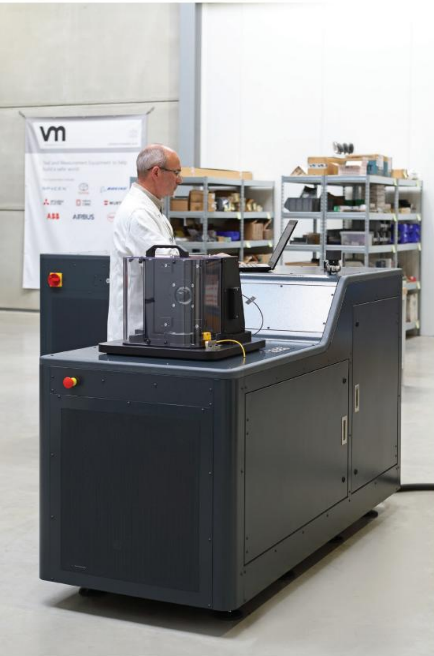
Figure 4: Vibration test equipment that can deliver closed-loop controlled transverse shear force and includes the inner joint surface friction correction factor and the option of using the same materials specified in the original bolted joint design clamped directly together.
