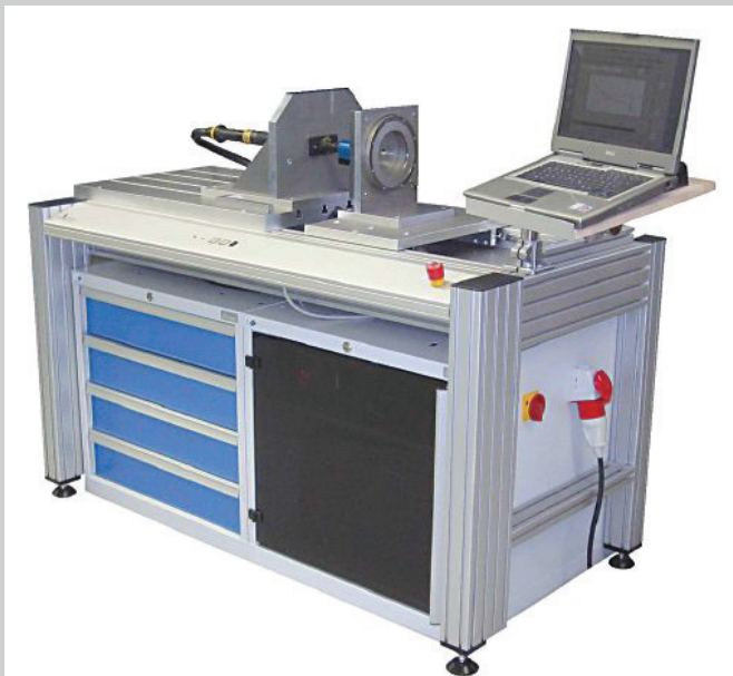
A fastener analysis system, FAST 500, with an electronically controlled driver unit and torque, rotation angle and clamp load measuring system (Source: REC®).
