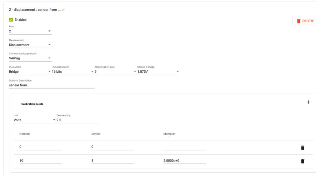
The second element allows the user to enable or disable the sensor:
