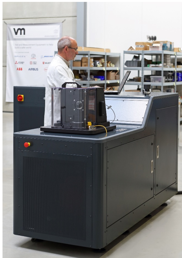
Vibrationmaster's J600 and J900 models offers real-time controlled transverse shear force load testing
